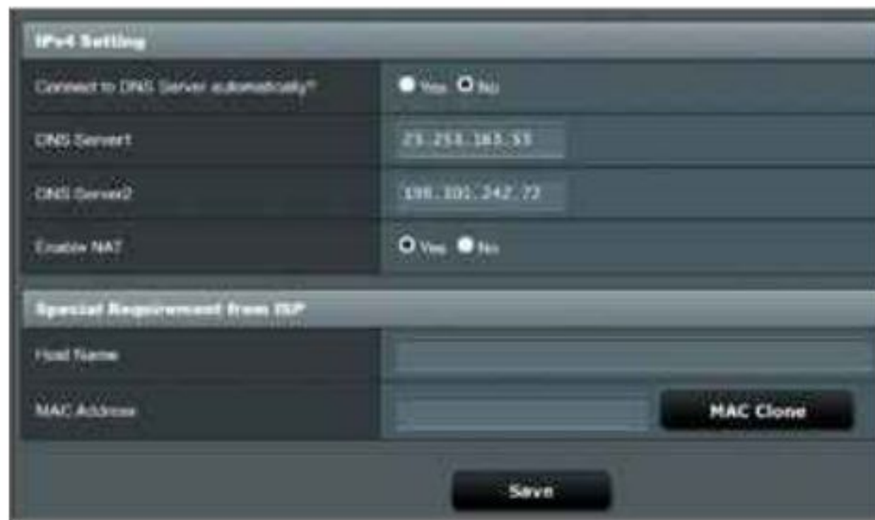
Change your DNS server to Alternate DNS to block ads and malware at router level
