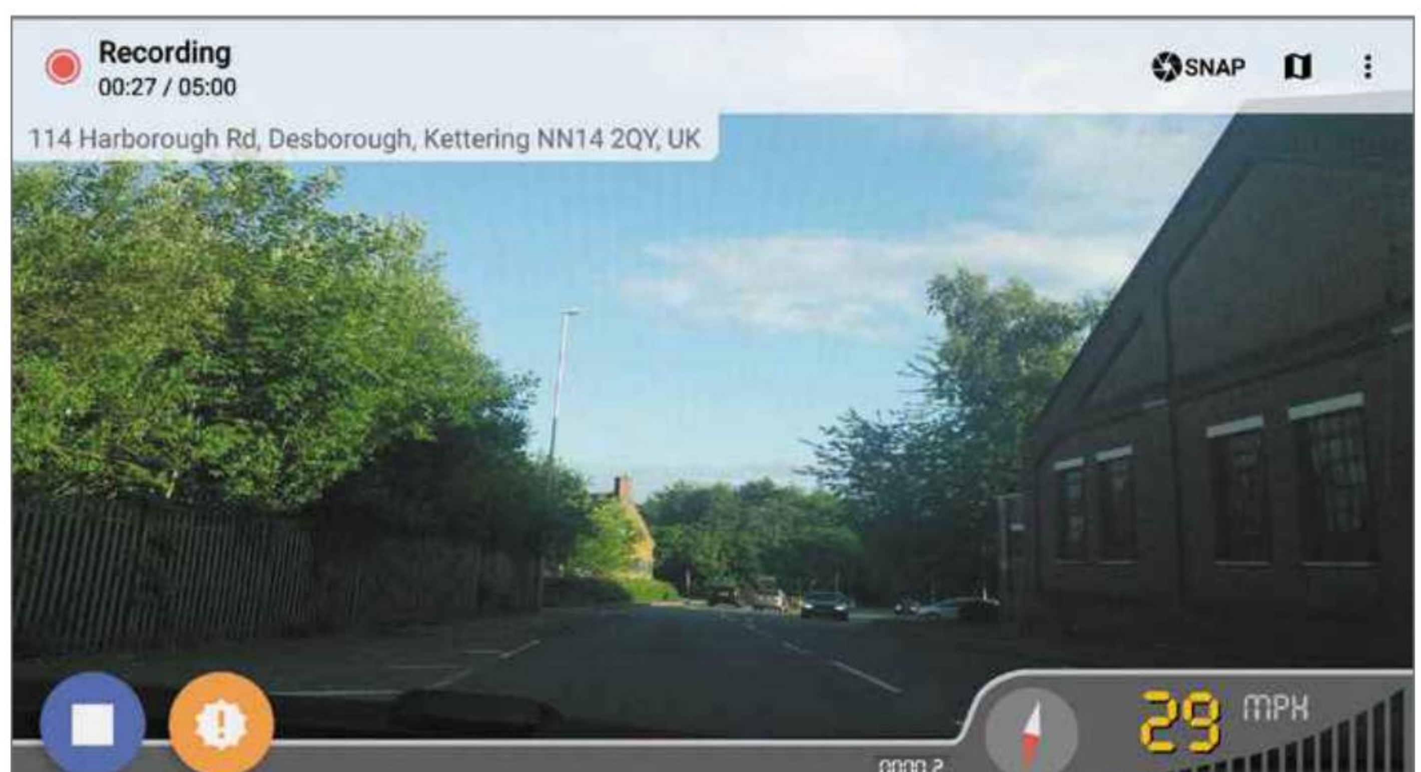
Tap the exclamation mark in AutoGuard to save the current recording as an accident video and optionally contact the emergency services
